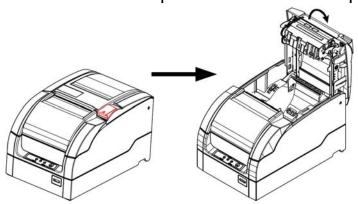
2) Hold the hole in the paper guide to rotate upward and disassemble it. When using 76mm, 69mm, 57mm width paper roll, user needs to insert paper guide vertically into a suitable location. When using 80mm paper roll, the paper guide will not be used, please keep the paper roll well.
