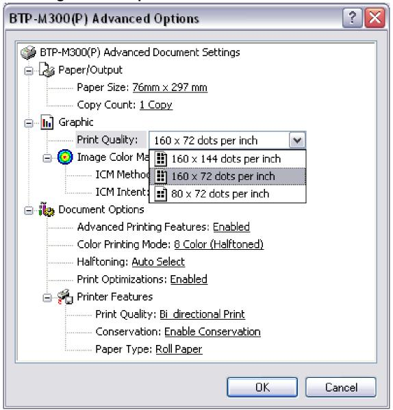
BTP-M300 driver supports three kinds of resolutions: 160 x 144 dpi, 160 x 72 dpi, 80 x 72 dpi. Users can select it according to their own need. High resolution has clear printing while lower print speed; low resolution has higher print speed while less clear printing.
