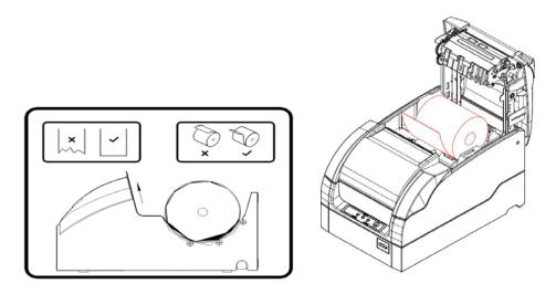
4) Pull out the paper head of paper roll along the paper feeding direction, close the rear cover, and tear off the surplus portion of the paper.
