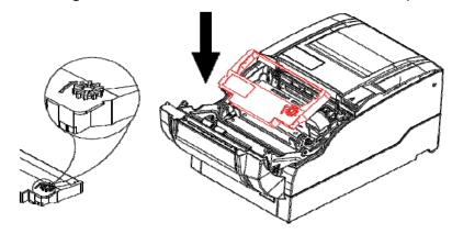
5) Turn the ribbon knob for two or three times according to mark to tighten the ribbon again.
